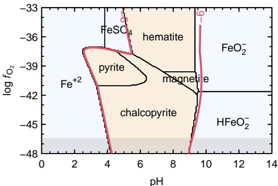
Stack 4: Cu minerals and aqueous  $\rightarrow$  Fe(Cu) minerals and Fe aqueous
